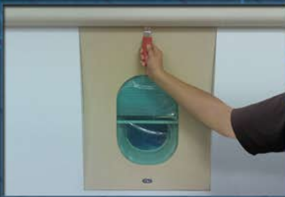
Electrical Shade Assy With Mechanical Override
